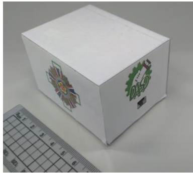
Figure 1. Appearance of inertial measuring device. Dimensions: 7.3×5.4×4.3 cm. Approximate weight with batteries: 125 g.
